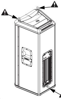
Before installing the eyebolts, remove the rubber inserts protecting the enclosure's threads (HPR152i and HPR153i only).
